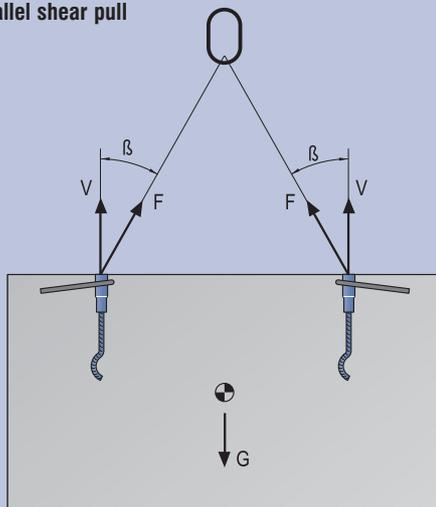
**4.6 Parallel shear pull and transversal pull with multi-legged sling sets**
