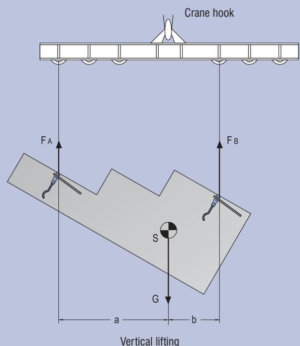
circumscribed by the anchors, then all the anchors will bear the load, however to different degrees. In simple cases, the different anchor forces can be calculated by two anchors on the head side or by three anchors on the surface of a panel. For this purpose, point 4.5 must be taken into account.
