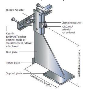
Figure 1: Brickwork support bracket with cast-in anchor channel
