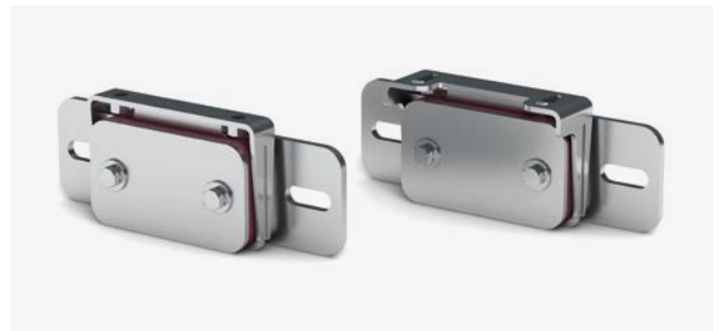
Modification of the JAI types to create dowel variant If it is not possible to secure the JAI elements to anchor channels, custom-designed dowel variants of the elevator insulation JAI can be used. The JAI element is pre-fitted on a dowel plate and then fixed in the shaft with dowels.
