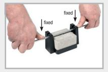
Pushing the wire through into the lower mount. The wire is permanently locked in place.
