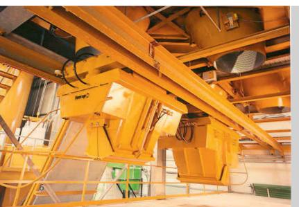
Special, duo-rail tandem concrete travelling buckets type 1000 + 2200 for travelling in curves.
