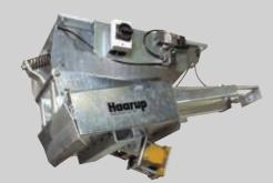
Combined batching gate for large quantities and vibration channel for fine batching.
