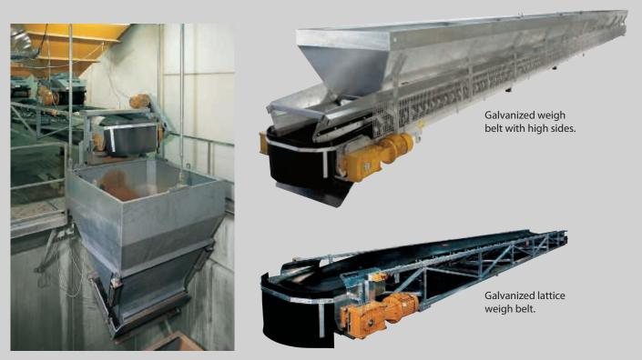
Combined weighing system with lattice weigh belt and weigh hopper.
