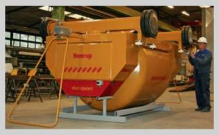
3500 litre duo-speed concrete travelling bucket is beeing tested before delivery.
