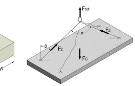
The slab unit has the following dimensions: L = 5 m w = 2 mt = 0.2 m
