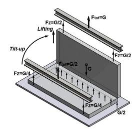
Lifting the walls from horizontal to vertical position without tiltup table.
