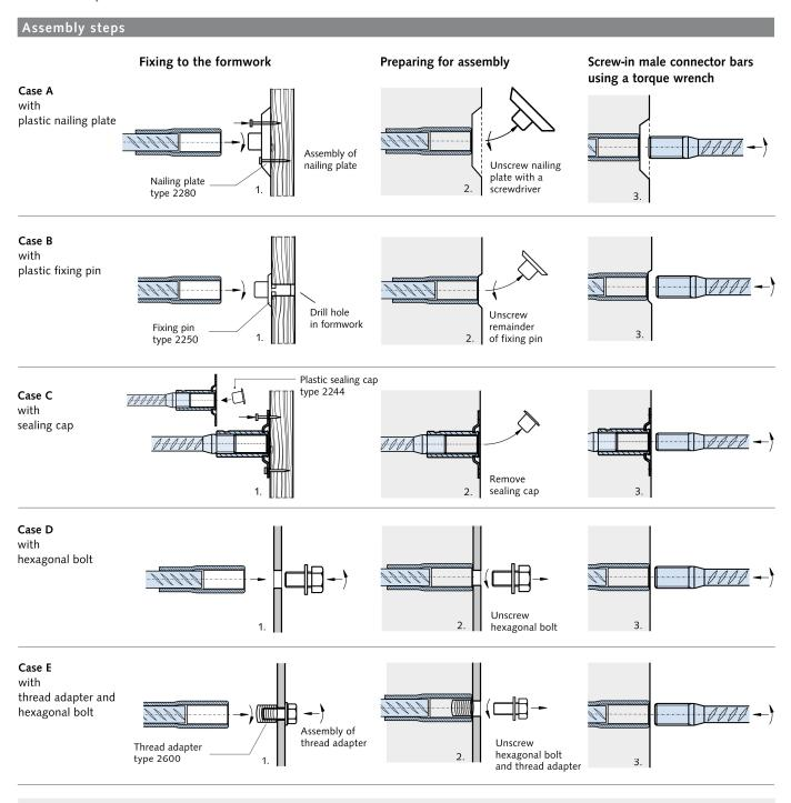
The female socket bars and male connector bars must be stored so that they remain free of dirt to ensure both can be easily connected. For further protection against ingress of dirt and concrete sludge, we also advise greasing the inside of the sleeve. Male connector bars should be tightened using a torque wrench set to the correct torque value.
