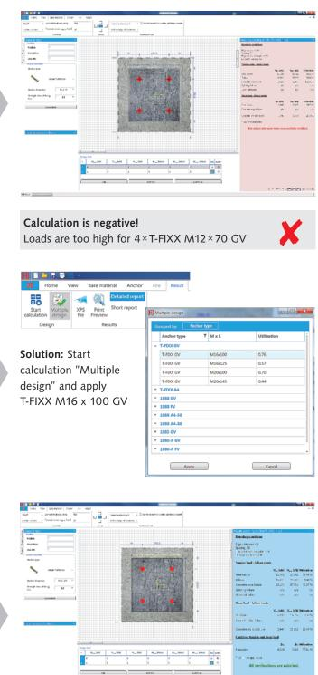
Calculation is positive with  $4 \times T$ -FIXX M16  $\times$  100 GV
