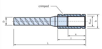
The sleeve has a metric ISO thread and is made of stainless steel (strength class A4-80).
