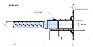
The sleeve is zinc galvanized (GV), the internal thread is metric ISO.
